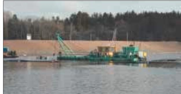
The dredging of the Bay of Örserum started in April 2002. The operation is carried out from a dredger that carefully sucks up the sediment. The slurry is pumped on shore through a buoyant pipe.
